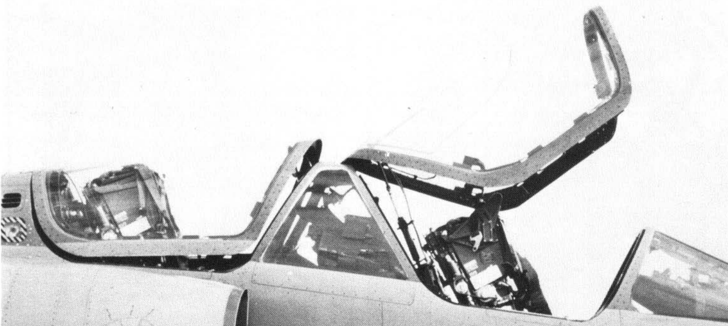
The two-seat training variants of the "Mirage F1", such as this "F1B", are equipped with an extended plexiglas canopy that accommodates the needs of both front and back seat occupants. Forward view requirements dictate that two-seat "Mirage F1's" have a taller transparency area than single-seat aircraft. Additionally, a fixed transparency section is mounted between the two crew stations to accommodate the side vision requirements of the back seat crew member.
