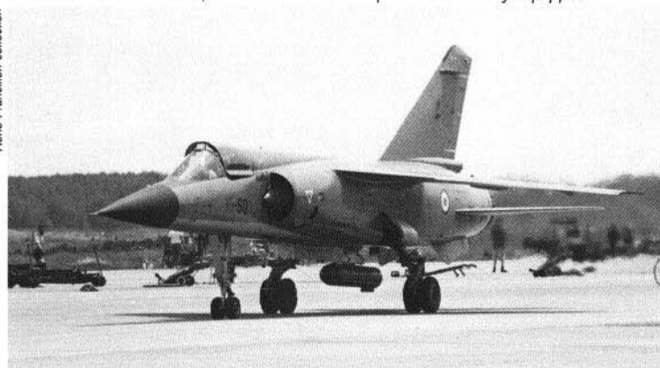
"Mirage F1C", 10-SQ, of E.C. 1/10 "Valois", taxis out on a training mission from Solanzara air base. The aft-mounted store is a SECAPEM 90 target towing container attached to an ALKAN 910 centerline pylon.
