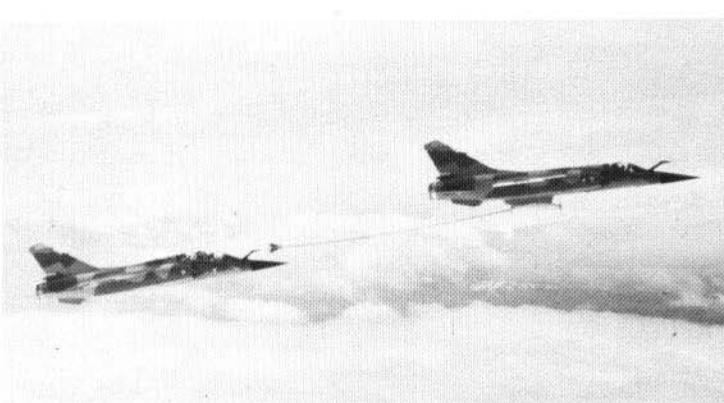
The "Mirage F1" is capable of carrying an inflight refueling buddy pack that allows the aircraft to be used as an inflight refueling tanker. Fuel is apparently syphoned from onboard and external tanks and delivered to the receiver aircraft via the buddy pack. The buddy pack system is powered by a small, nose-mounted variable pitch propeller. The hose and drogue can be retracted or extended as required via the buddy pack reel and associated power supply.
