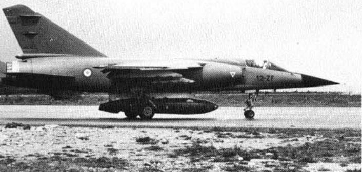
"Mirage F1C", 12-ZF, the 40th production "F1", of E.C. 3/12 "Cornouaille" has a single 1,200 liter centerline external fuel tank and two MATRA F4 unguided rocket pods suspended from ALKAN 910 and ALKAN 915 pylons, respectively.
