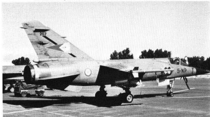
"Mirage F1C-200", 5-NP, of E.C. 1/5 "Vendée", during June, 1980. This aircraft is equipped with a pair of MATRA "Magic" AAM training rounds on its wingtip rails. 5-NP is the 207th production "Mirage F1".
