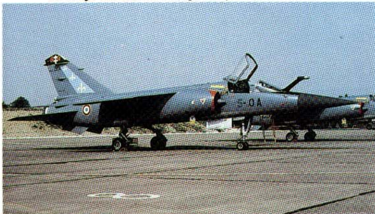
"Mirage F1C-200", 5-OA, of E.C. 2/5 "Ile de France". All flight refueling probes seen on "F1C-200" series aircraft are painted black in order to eliminate distracting glare.
