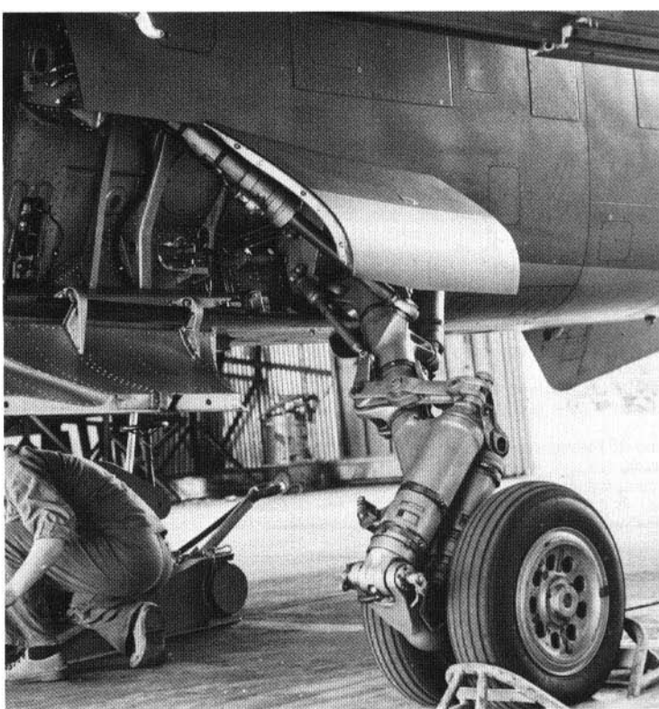
The "Mirage F1's" main gear assembly is perhaps the single most complex structure in the aircraft. It is designed to be both exceptionally rugged and amazingly versatile, and it permits the aircraft to operate from a variety of surfaces while carrying many different payload types and sizes. The retraction sequence, explained in more detail on page 32, is extraordinarily complex; it requires the main gear to rotate as they retract.
