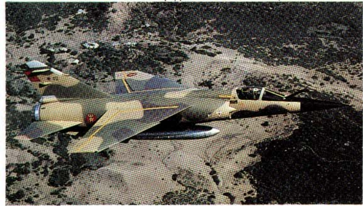
"Mirage F1EH-200", No. 172, of the Royal Moroccan Air Force during December, 1980. Markings are standard for RMAF aircraft. The wing warning stripes are noteworthy, as is the 1,200 liter centerline drop tank.
