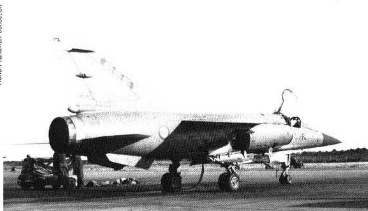
"Mirage F1C", 30-FL, of E.C. 3/30 "Lorraine" at the Solenzara air base (B.A. 126). An electrical system power cart is attached to the aircraft for start-up. Markings are standard for type.
