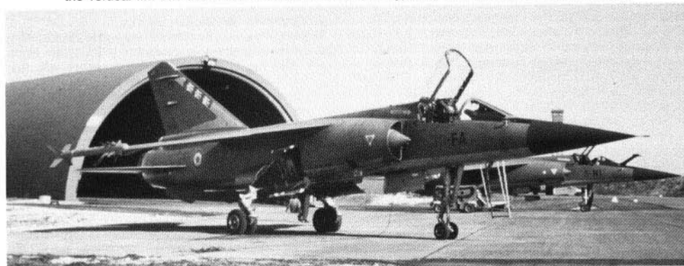
A "Mirage F1C" of E.C. 3/30 mounting two MATRA 550 "Magic" short range air-to-air missiles on its wingtip rails. Visible in the background is the aircraft's hardened protective shelter, typical of such facilities throughout Europe. The E.C. 3/30 vertical fin patch is readily discernible.
