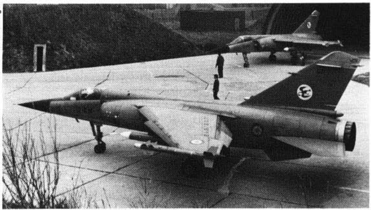
"Mirage F1C's", 12-KN and 12-KG, of E.C. 1/12 "Picardie". Both aircraft are armed with MATRA "Super 530 F" AAM's on their wing pylons and MATRA 550 "Magic" AAM's on their wingtip rails.
