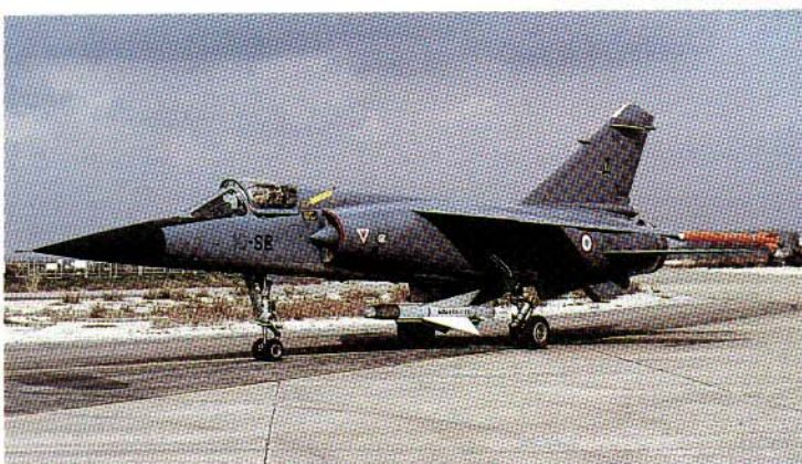
"Mirage F1C", 10-SB, of E.C. 1/10 "Valois". It is equipped with a single MATRA R 530 air-to-air missile on its centerline pylon, and the French equivalent of an AIS (Aircraft Instrumentation Subsystem) pod on its left wingtip rail.
