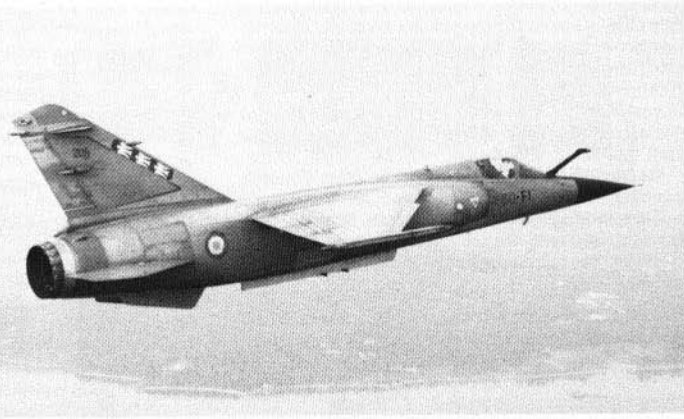
"Mirage F1C-200", 30-FI, of E.C. 3/30 "Lorraine" over Corsica during a practice intercept mission. This aircraft is equipped with an ALKAN 910 centerline pylon and two wingtip missile rails.
