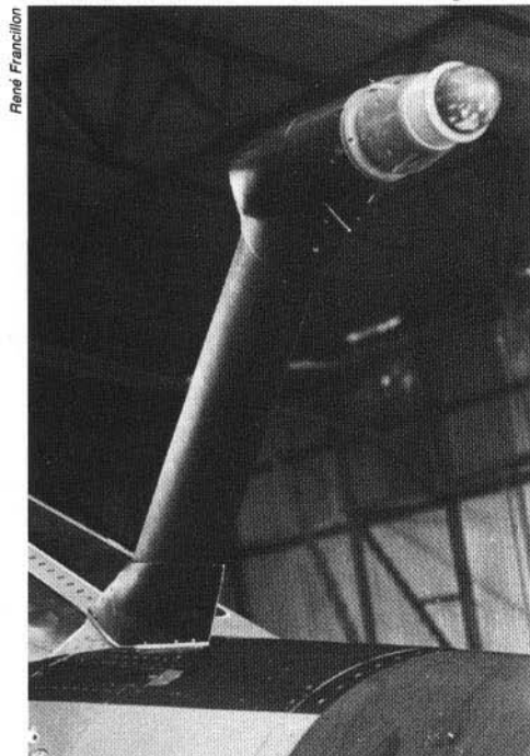
The inflight refueling probe, when it was installed as a modification on older production "Mirage F1C's", entailed a nose plug insert, thus increasing the aircraft over-all length. To accommodate the forward vision requirements of the pilot, the probe was designed to be offset to the right side of the aircraft. The probe's male fitting is standardized for use with all U.S. and European and NATO inflight refueling tankers.
