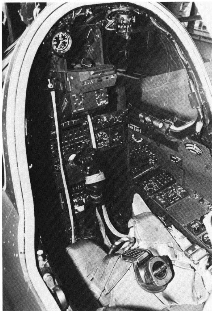
The "Mirage F1" cockpit is small by American standards, but none the less adequate. Front panel and console layouts are efficient and easily accessed. Most of the instrumentation is analogue, though some digital indicators are visible.
