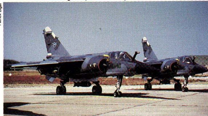
Two "Mirage F1CR's", 33-ND and 33-NG, of E.R. 2/33, "Savoie", are seen with each carrying three 250 kg. SAMP general purpose iron bombs. Two bombs are mounted on ALKAN M2 wing pylons and one on an ALKAN 910 centerline pylon.
