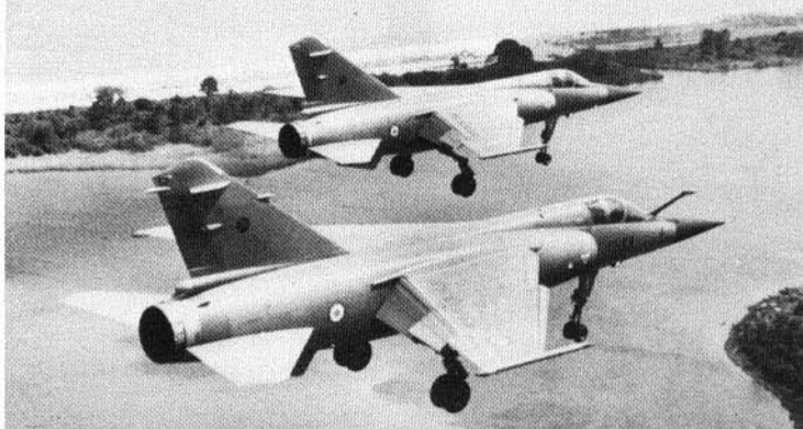
"Mirage F1C-200", 12-KA, and a "Mirage F1C", 12-KC, of E.C. 2/12 "Picardie", are seen on final approach over the Mediterranean Sea. Differential deployment of both flaps and flaperons is readily apparent.
