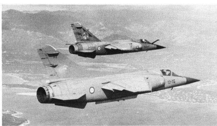
"Mirage F1C", 12-YG (foreground), and "Mirage F1C-200", 12-YT, both of E.C. 1/12 "Cambrésis", practice formation maneuvers in October, 1983. 12-YG is flying with an ALKAN 910 centerline pylon, though no store is carried.
