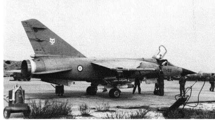
"Mirage F1C", 10-SU, of E.C. 1/10 "Valois". This is the 10th production "Mirage F1", and like 10-SW, it is carrying a telemetry pod on its right wingtip rail. an R 530 AAM is mounted on an ALKAN 910 centerline pylon.
