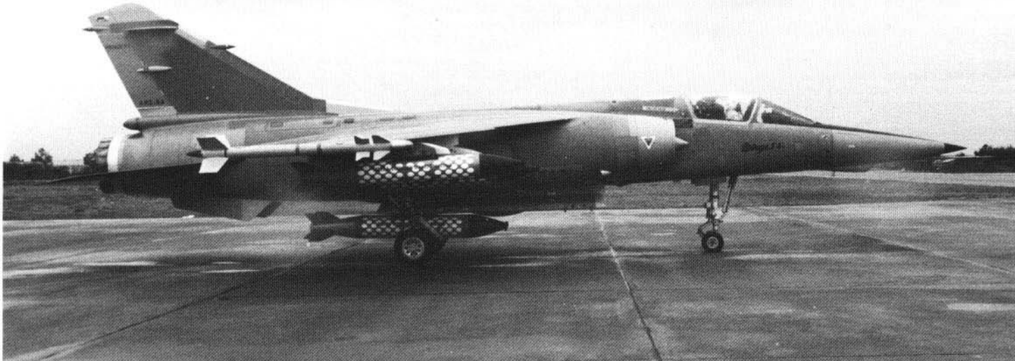
A prototype "Mirage F1" is seen carrying a load of six MATRA-BRANDT "Bélouga" grenade launchers and two MATRA R 550 "Magic" AAM's. Each "Bélouga" pod carries 166 2.65 lb. grenades which can be sequentially ejected over target areas leaving a rather large path of destruction. The small grenades are forcibly ejected from the pod via small pyrotechnic charges. The grenades descend by parachute, exploding upon ground contact.
