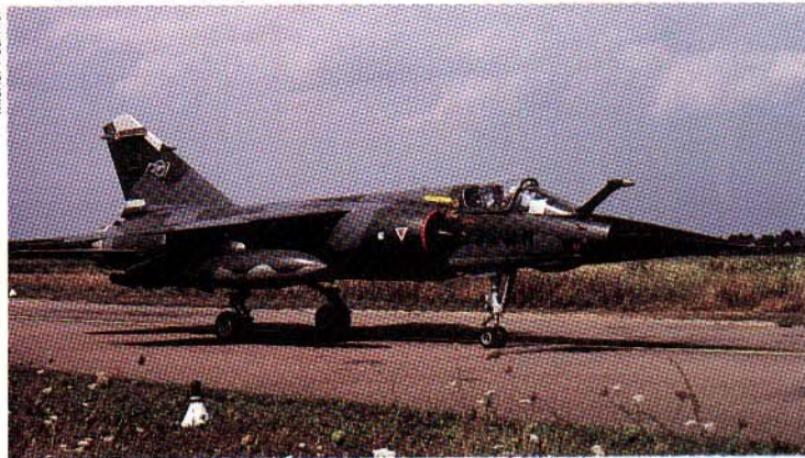
"Mirage F1CR", 33-NN, of E.R. 2/33 "Savoie", during August, 1985. This is one of the most recent "Mirage F1CR" deliveries and it bears the latest "Armée de l'Air" camouflage pattern. The unit badge is readily visible on the vertical tail fin.
