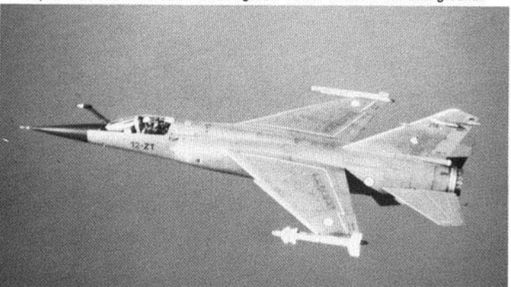
"Mirage F1C-200", 12-ZT, the 254th production "F1", of E.C. 3/12 "Cornouaille", during a practice sortie with a MATRA R 550 "Magic" visible on the left wingtip rail, and a French AIS pod equivalent visible on the right wingtip rail.
