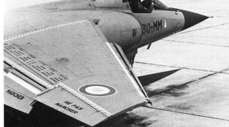
An excellent view of the "Mirage F1" upper wing surface showing the outer panel leading edge slat, the inner panel leading edge flap, the slotted flaps, the flaperons, and the rarely noted spoilers. The slats and flaps have been extended.
