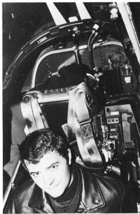
The "Mirage F1" ejection seat headrest and rear cockpit. Like other aspects of "F1" design and construction, this area is neatly executed.
