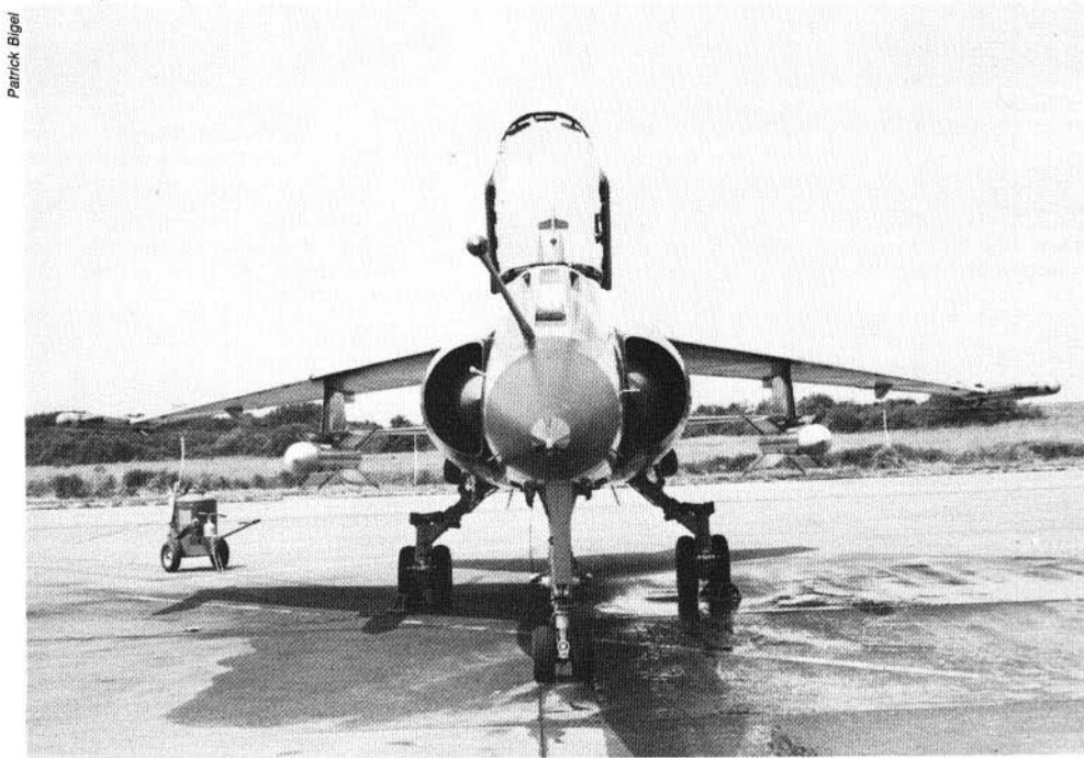
The inflight refueling probe, when it was installed as a modification on older production "Mirage F1C's", entailed a nose plug insert, thus increasing the aircraft over-all length. To accommodate the forward vision requirements of the pilot, the probe was designed to be offset to the right side of the aircraft. The probe's male fitting is standardized for use with all U.S. and European and NATO inflight refueling tankers.
