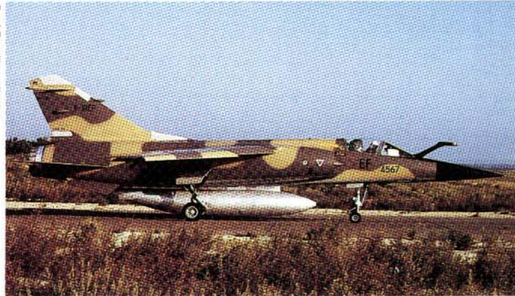
"Mirage F1EQ", No. 4567, of the "Al Quwwat al Jawwiya al Iraquiya" (Iraqi Air Force). It is seen with a long-range 2,200 liter centerline drop tank that is normally used only for long range ferry missions.
