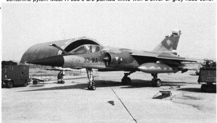
"Mirage F1CR", 33-NA, the 603rd production "F1", of E.R. 2/33 "Savoie". The reconnaissance camera bay is located just ahead of the nose gear and is visible in the form of a ported fairing, or bump.
