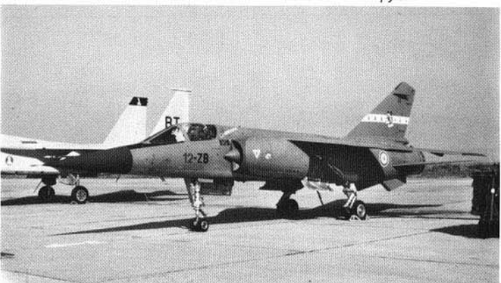
"Mirage F1C", 12-ZB, the 19th production "F1" of E.C. 3/12 "Cornouaille", during a practice sortie with a MATRA R 550 "Magic" visible on the left wingtip rail, and a French AIS pod equivalent visible on the right wingtip rail, in September, 1981. A McDonnell Douglas F-15A is visible in the background.
