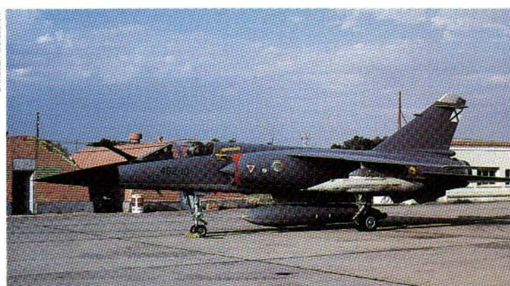
"Mirage F1EE", C.14B-61, of Escuadrón 462, Mando Aéreo de Canarias, Ejército del Aire, at Zaragoza-Valenzuela, during May, 1985. It carries a single 1,200 liter centerline drop tank and two wing mounted DEFA 30mm gun pods.
