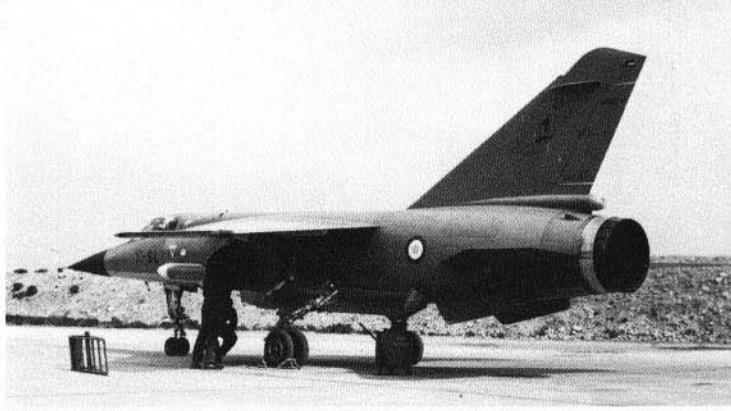
"Mirage F1C", 10-SL, of E.C. 1/10 "Valois", prior to taxiing out on a training mission while carrying a MATRA "Super 530" AAM on its left wing pylon. The "Super 530" is a much improved development of the original R 530 AAM.
