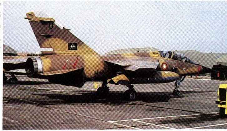
"Mirage F1DDA", QA 62 "U", of the Qatar Emiri Air Force, at Orange-Caritat, France, during February, 1984. The Middle-Eastern camouflage is typical of QEAF aircraft. Noteworthy is the camouflaged 1,200 liter drop tank.
