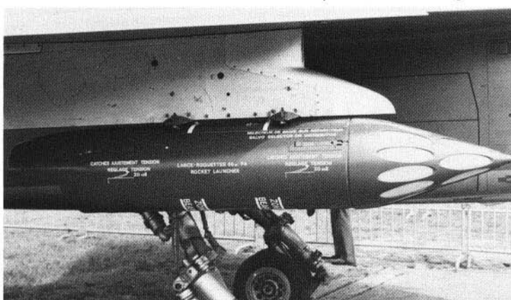
MATRA F4 68mm rocket launchers can be attached to the "Mirage F1" using an ALKAN 915 wing pylon. Each of these launchers carries a total of 18 68mm air-to-surface solid fuel fin-stabilized rockets which are salvo launched against targets as necessary. The rockets are loaded from the rear of the pod. Frangible plastic fairings fill the forward pod exits, these disintegrating as the rockets are ignited and propelled forward.
