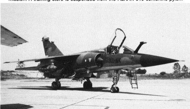
"Mirage F1CR", 33-NK, the 613th production "F1", of E.R. 2/33 "Savoie". Two MATRA F4 unguided rocket pods are suspended from the wing pylons, verifying that the "F1CR" can be used for ground support work as well as recce.
