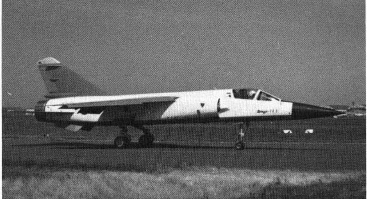
Most powerful "F1" version to reach the hardware stage was the "F1E". Powered by a SNECMA M.53 rated at 18,740 lb. th., it was pitted unsuccessfully against the YF-16 and YF-17 in what was billed as the "Deal of the Century".
