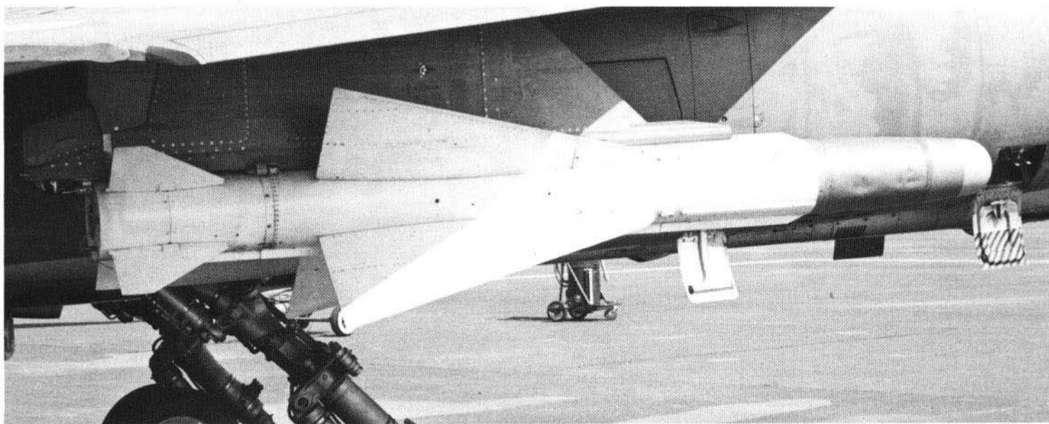
The MATRA R 530 is normally painted white with the sensor head painted silver or some other light color. A removable cap normally protects the infrared sensor receiver and associated glass dome when the aircraft is sitting statically. The R 530 is normally carried under the "Mirage F1" using a Type 38DN pylon. It is possible for the "Mirage F1" to carry up to three R 530's at one time.
