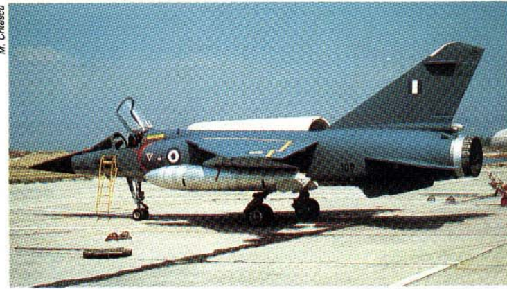
"Mirage F1CG", No. 109, of 114a Pterix Mahis, of the "Helliniki Aeroporia" (Greek Air Force), during August, 1975. It is equipped with a pair of 1,200 liter drop tanks.
