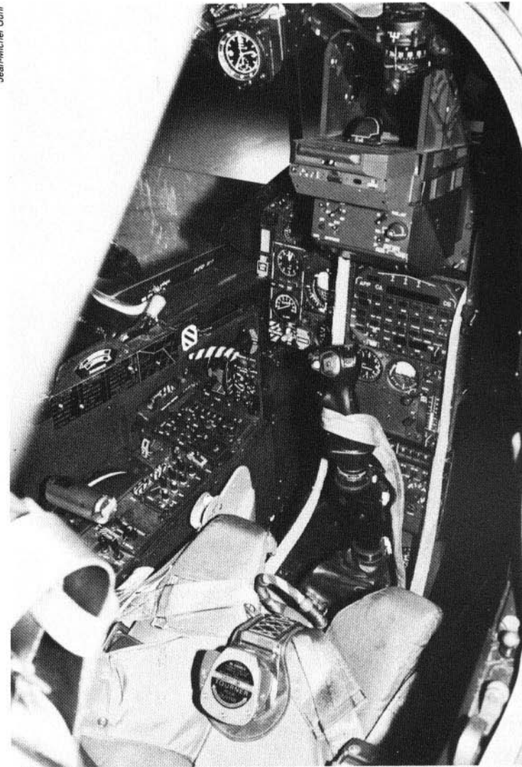
The large, centrally-mounted HUD takes up most of the "F1's" upper instrument panel space. Most of the standard flight instruments are located on the left, lower center, and right panels of the conventional T-shaped forward instrument panel.
