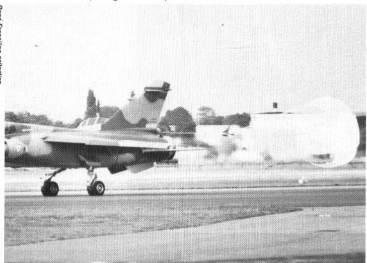
A camouflaged "Mirage F1B" is seen (rt.) with its large drag chute deployed, immediately following landing. The drag chute is housed in a bullet fairing situated just above the empennage section with the chute deployment door mounted just above the engine exhaust nozzle. The bullet fairing is known to have been used on occasion to house an advanced, but unidentified electronic countermeasures unit working in conjunction with a set of wing-mounted ECM pods.
