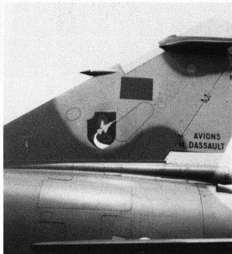
The "Mirage F1" empennage and vertical fin are provided with a significant number of removable panels to accommodate maintenance needs.
