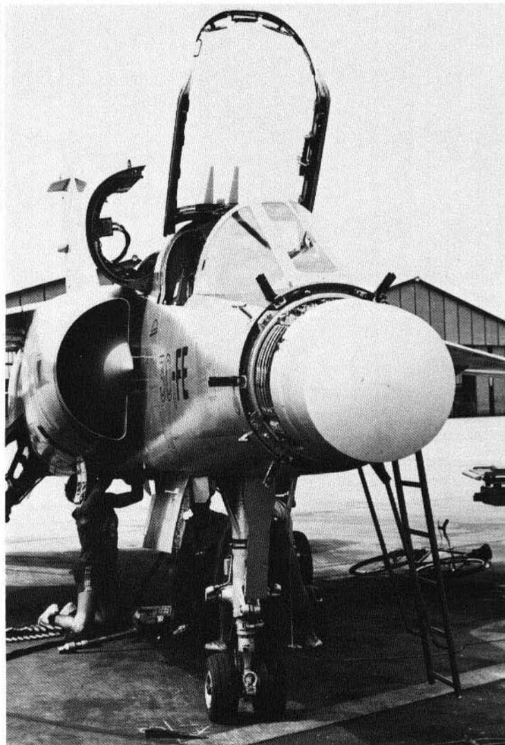
The "Mirage F1C's" Thomson-CSF "Cyrano IV" radar is a monopulse, I/J-band set employing a cassegrain scanner. It is utilized in several variations by the "F1", and in more advanced units has a limited look-down capability.
