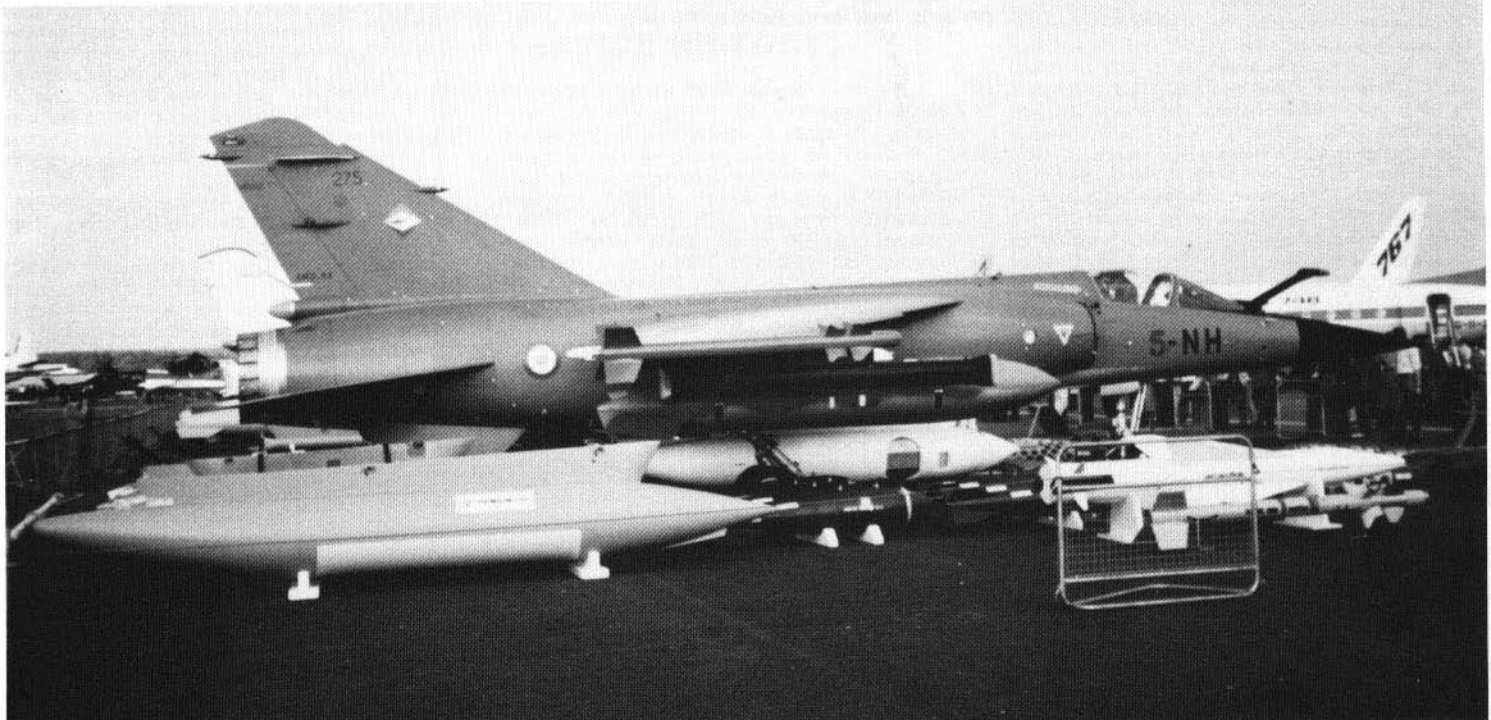
"Mirage F1C", 5-NH, of the "Armée de l'Air" poses at a Paris Airshow with a selection of the weapons, ECM pods, fuel tanks, and reconnaissance pods which it is capable of carrying. Of particular interest is the large Thomson-CSF side-looking airborne radar pod in the foreground, and the Thomson CSF DB3163 electronic countermeasures pod mounted on the right inboard wing pylon. Also notable is the reconnaissance pod located near the center of the display.
