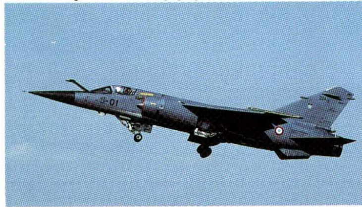
"Mirage F1C-200", 5-OI, of E.C. 2/5 "Ile de France". It is seen shortly after lift-off with the landing gear in mid-retraction. The rotational geometry requirement of the main gear is noteworthy.
