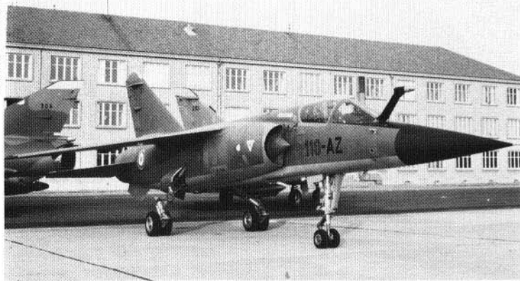
"Mirage F1C-200" of the C.E.A.M. Built as the first production "Mirage F1C", it later became the first aircraft brought up to the "F1C-200" standard. The C.E.A.M. operates several variants of the "Mirage F1".
