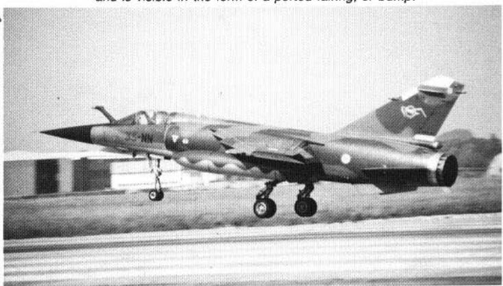
"Mirage F1CR", 33-NN, the 616th production "F1", of E.R. 2/33 "Savoie", landing following a training sortie. The aircraft is equipped with a jettisonable 1,200 liter (317 gals.) external fuel tank under each wing.
