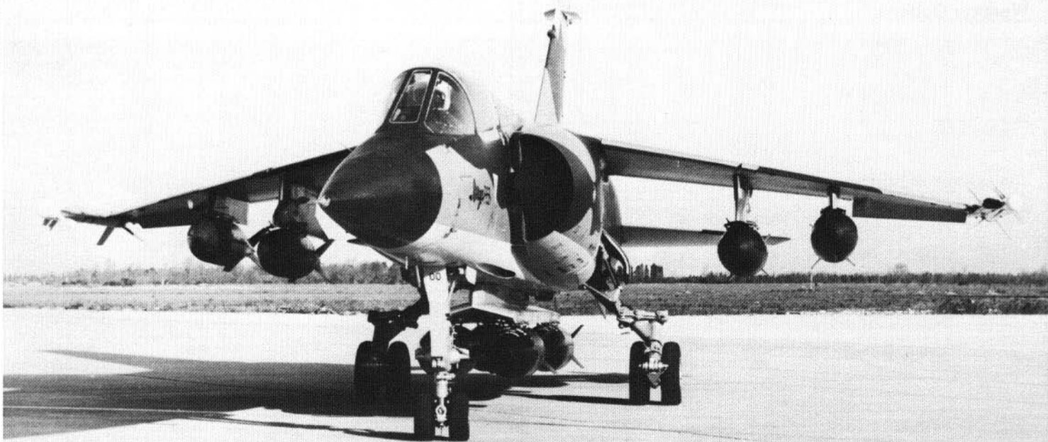
Almost certainly operating at or near its maximum payload capacity, a South African Air Force "Mirage F1CZ" is seen carrying no less than eight 400 kg. (881 lbs.) iron bombs on various ALKAN pylons. Mounted on the wingtips are two MATRA R 550 "Magic" AAM's. The "F1" has been used as a ground support aircraft in actual combat and has proven itself to be well adapted to the role. Note extended flaperons.
