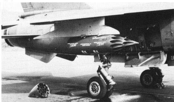
MATRA F4 68mm rocket launchers can be attached to the "Mirage F1" using an ALKAN 915 wing pylon. Each of these launchers carries a total of 18 68mm air-to-surface solid fuel fin-stabilized rockets which are salvo launched against targets as necessary. The rockets are loaded from the rear of the pod. Frangible plastic fairings fill the forward pod exits, these disintegrating as the rockets are ignited and propelled forward.
