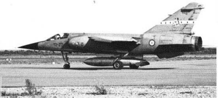
With its 1,200 liter centerline external tank seemingly dragging the taxiway, "Mirage F1C", 12-ZD, the 82nd production "F1", of E.C. 3/12 "Cornouaille", taxis out on a practice sortie from the Solenzara air base (B.A. 126).
