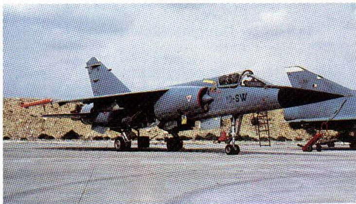
"Mirage F1C", 10-SW, of E.C. 1/10 "Valois". The French equivalent of an AIS (Aircraft Instrumentation Subsystem) pod is seen on its right wingtip rail. The AIS is part of the ACMI (Air Combat Maneuvering Instrumentation) system.
