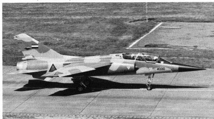
An Iraqi Air Force "Mirage F1BQ-1" two-seat trainer. This particular example, assigned Iraqi Air Force serial number 4000, was the first two-seat "Mirage F1" variant delivered to Iraq.
