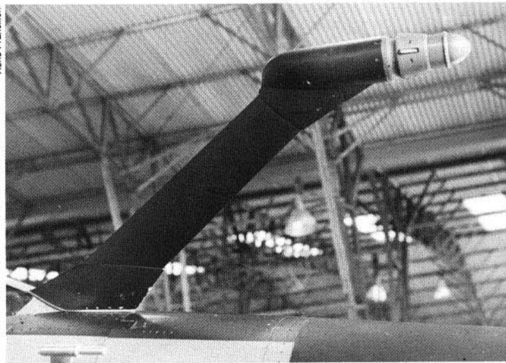
The refueling probe, which delineates the "Mirage F1C-200" from the standard "F1C", has been retrofitted to a number of early production aircraft. Late production samples have been manufactured with the probe as a standard feature.
