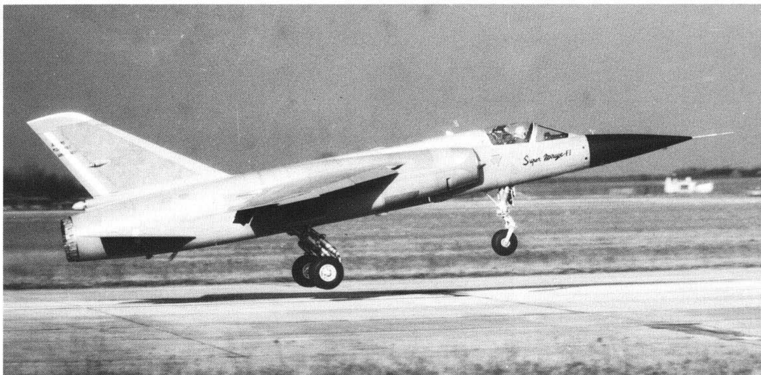
The prototype "Mirage F1", at the time referred to as the "Super Mirage F1", flares for landing at the "Centre d'Essais en Vol" Brétigny test facility during the course of its preliminary flight test program. Of particular interest in this photo is the single-wheel nose gear—later replaced with the dual-wheel unit seen on all production "F1's". This aircraft was lost on May 19, 1967, while practicing an aerobatic routine for the Paris Airshow.
