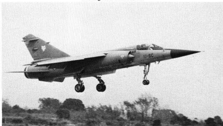
"Mirage F1C", 10-SC, of E.C. 1/10 "Valois", is seen moments before touching down at the Solanzara air base. Worthy of note are the lowered leading edge flaps, the lowered trailing edge flaps, and the aircraft's mild pitch attitude.
