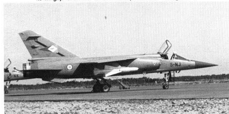
"Mirage F1C", 5-NJ, of E.C. 1/5 "Vendée", at the Solenzara air base (B.A. 126). It is carrying a MATRA R 530 infra-red guided AAM on its starboard wing pylon. The distinctive E.C. 1/5 vertical fin art is readily apparent.
