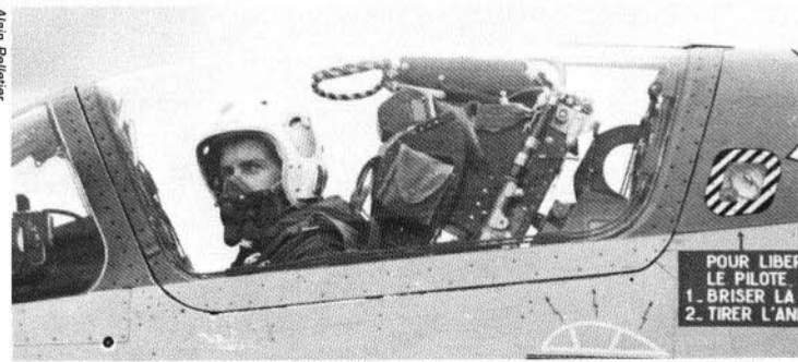
The "Mirage F1" cockpit is dimensionally small. The canopy configuration is conventional and utilizes a single hydraulic ram for opening and closing. The ejection seat can be actuated by using either standard hand grips or the overhead pull rings. Visible in photo on left is the emergency egress knife (with barber pole handle) attached to the canopy frame. This can be used by the pilot to break the canopy plexiglas in case other forms of canopy removal fail.
