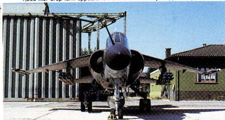
A "Mirage F1CR" with twelve BRANDT BAP 100 parachute-retarded bombs mounted on ALKAN M2 wing pylons under each wing. The BAP 100 is considered a "cratering" weapon and is designed for runway destruction.
