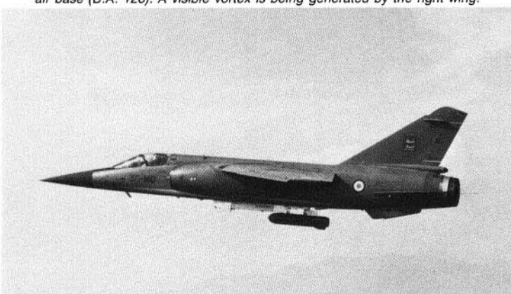
"Mirage F1C", 30-MO, the 43rd production "F1", of E.C. 2/30 "Normandie-Nieman". The aircraft is seen flying out of Solanzara air base during a training mission. A training store is suspended from the ALKAN 910 centerline pylon.
