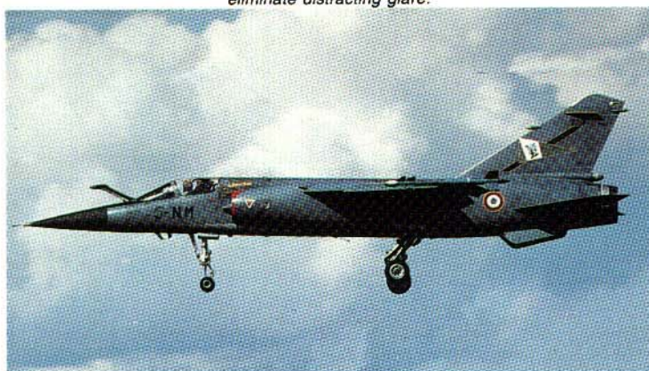
"Mirage F1C-200", 5-NM, of E.C. 1/5 "Vendée". It is configured for final approach and is seen landing at an unidentified French base on June 15, 1980. Extended nose gear strut and landing light (just ahead of strut) are noteworthy.
