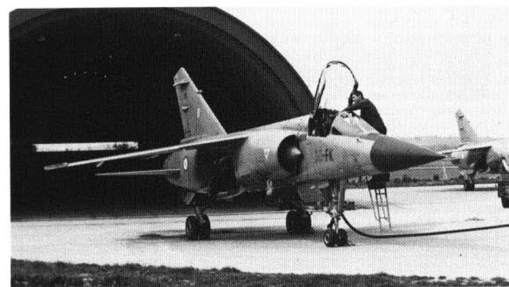
"Mirage F1C", 30-FK, of E.C. 3/30 "Lorraine" being fueled for a practice mission from its French base. The "Mirage F1" has a single-point refueling system. Hardened shelter in the background is of concrete and steel construction.
