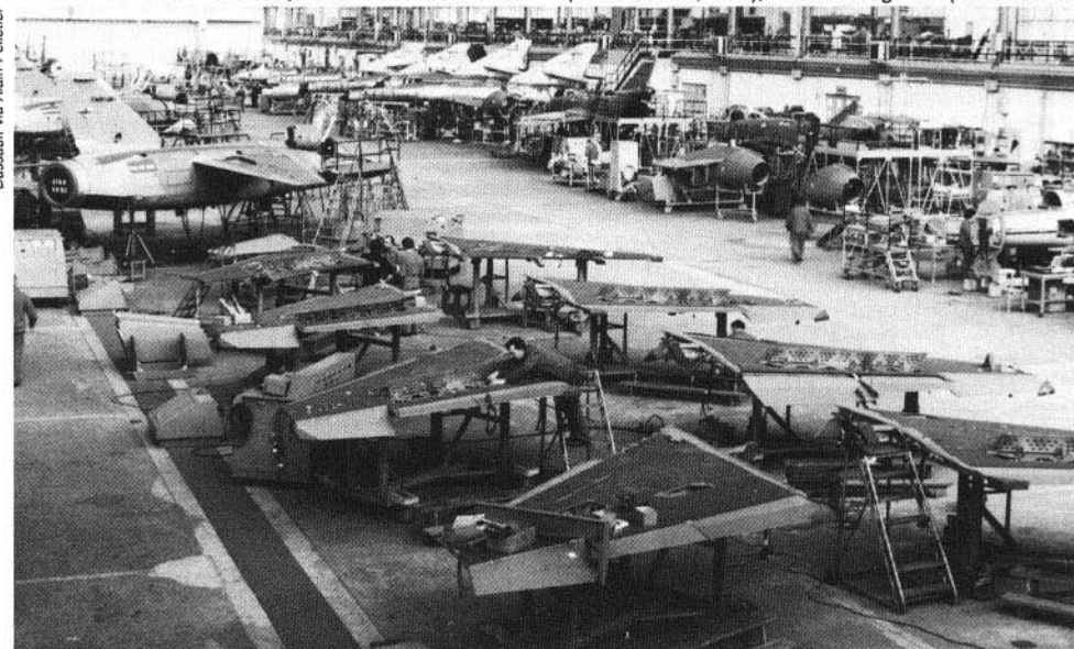
The "Mirage F1" production line at Dassault's Bordeaux plant was shared with a similar line for the "Super Etendard" carrier-based aircraft (background). Facilities do not appear to be as automated as contemporary U.S. facilities and there does not appear to be a true elevated production line process involved.
