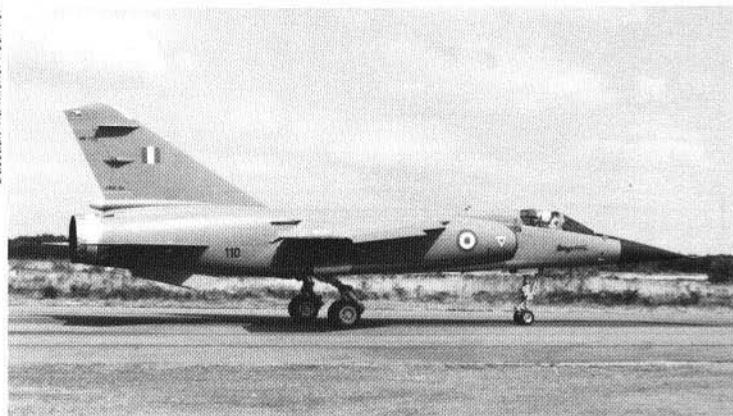
"Mirage F1CG", 110, of the Hellenic Air Force was one of 40 ordered from Dassault in June, 1974. The "F1CG" is basically similar to the "Armée de l'Air's" "F1C", but is modified to accommodate the AIM-9 "Sidewinder".
