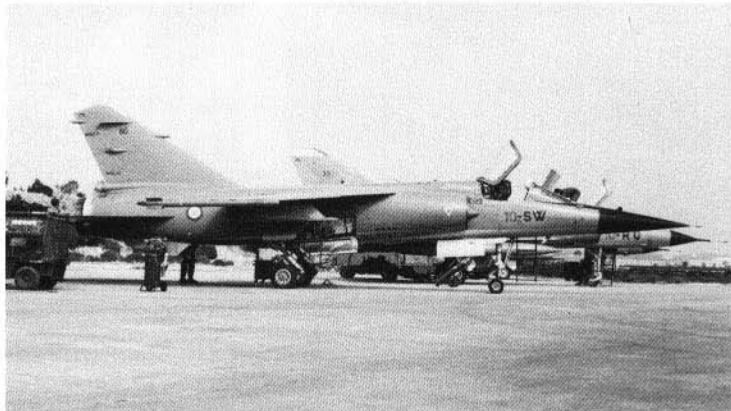
"Mirage F1C", 10-SW, of E.C. 1/30 "Valois". The 80th production "Mirage F1", it carries the French equivalent of an AIS (Aircraft Instrumentation Subsystem) pod. The AIS is part of a French ACMI system.
