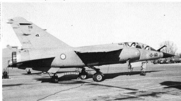
"Mirage F1B", 5-AR, of E.C. 3/5 "Comtat-Venaissin". This unit, consisting of ERC 571 and SPA 171, acts as an operational training unit and is equipped with both "F1C's" and "F1B's". Note the inflight refueling probe.
