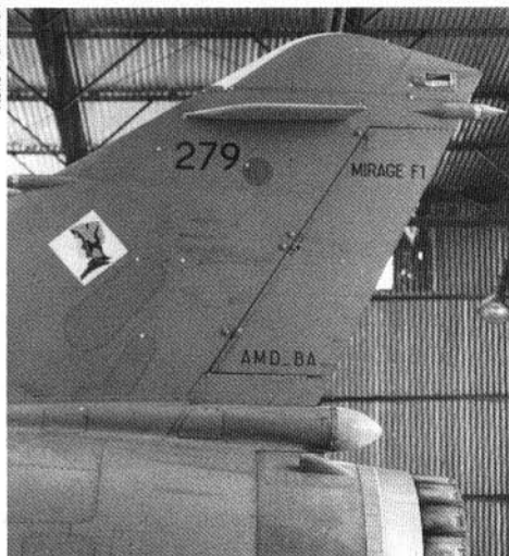
The "Mirage F1's" vertical fin is a conventional swept vertical surface with a single piece rudder. The rudder hinges are faired into the leading edge.
