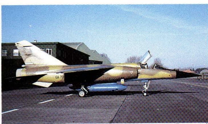
"Mirage F1EDA", QA 73, of the Qatar Emiri Air Force, with a centerline-mounted MATRA/Dassault "Harold" reconnaissance pod. At least two TV/camera configurations for this pod are known to exist.
